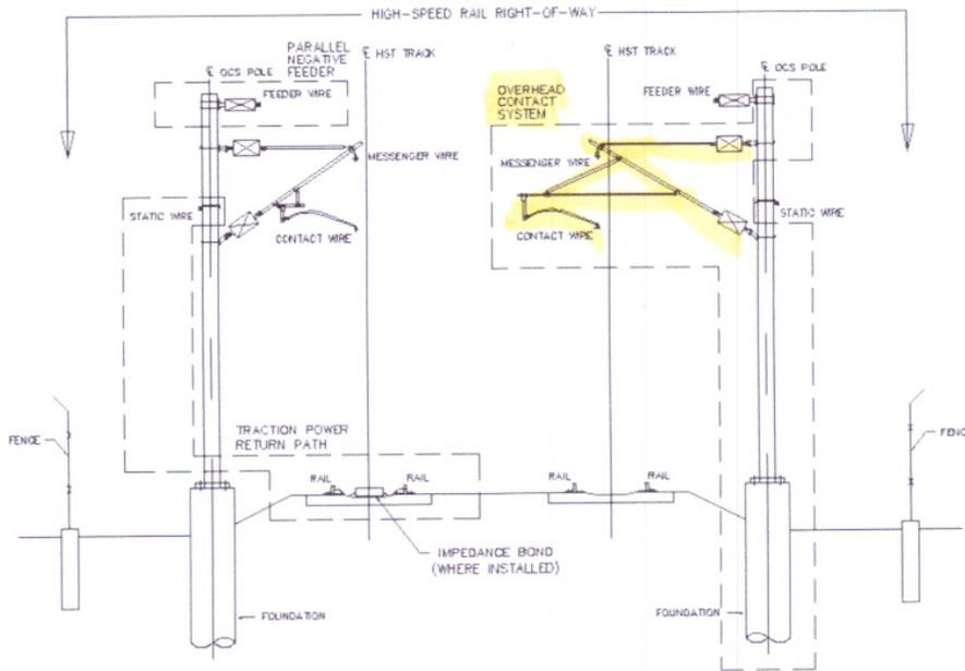
Figure 3-1 Typical 2x25 kV Electrification System
